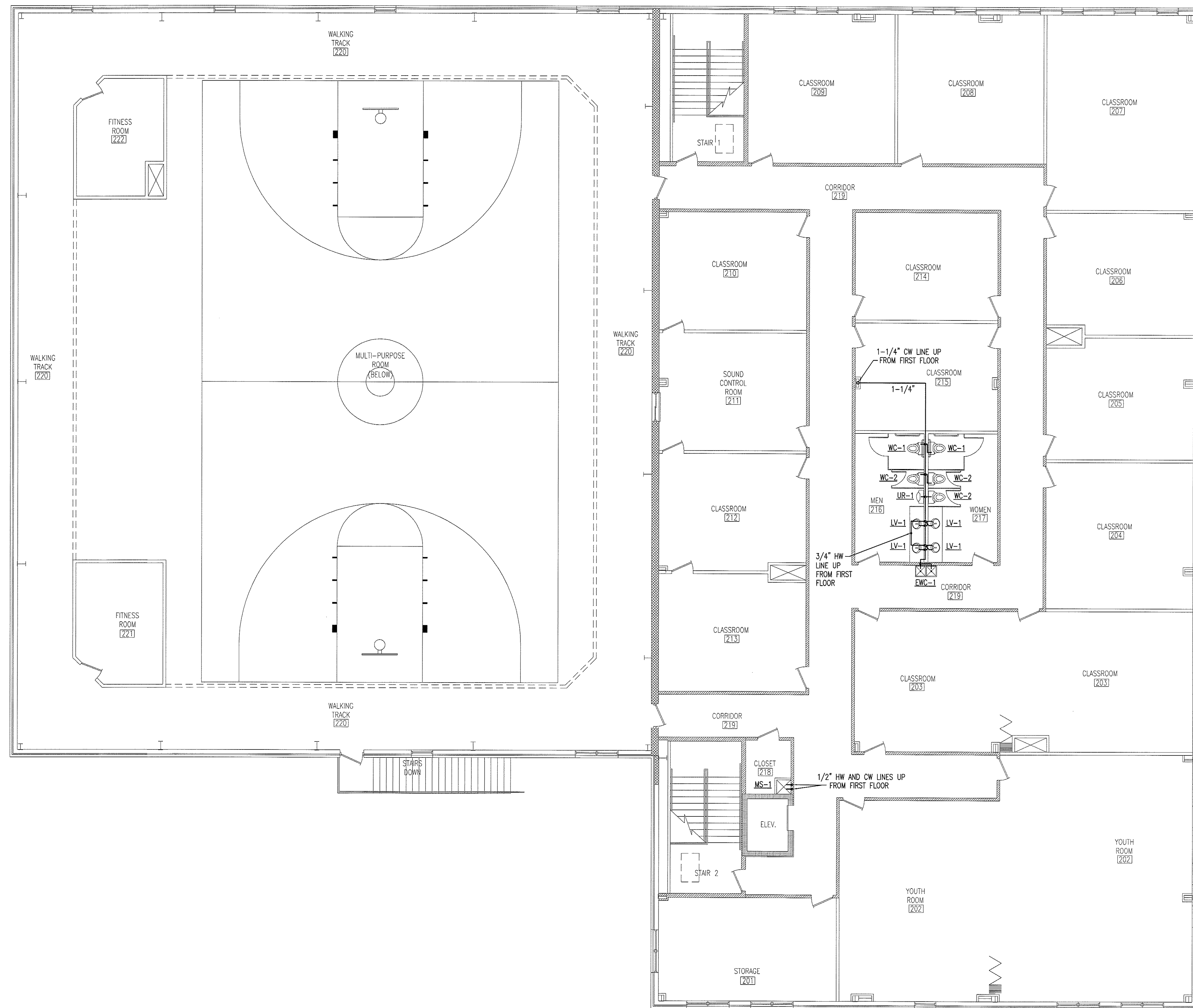
1 SECOND FLOOR WATER PIPING PLAN SCALE: 1/8" = 1'-0"
